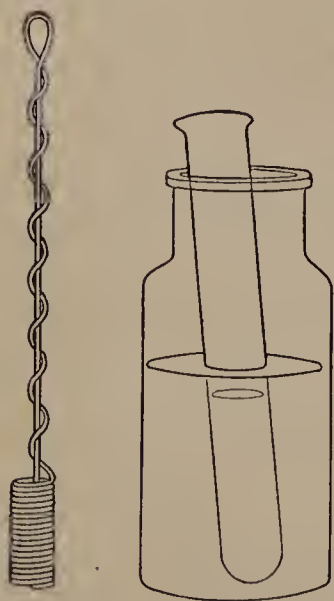
Fig. 83. Testing for methyl alcohol with a hot copper coil.
